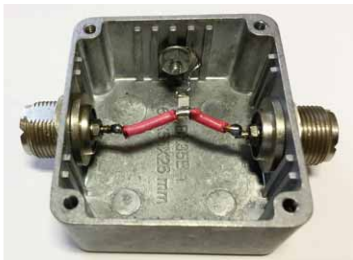
Figure 5 — This 80 m tuner uses a single capacitor.
