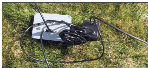
Figure 13 — Switching module, combiner amplifier and cabling for the enhanced array.
