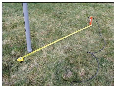
Figure 9 — Base of completed array showing link distance and loop splice.
